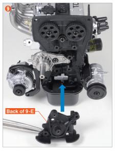
Fit the recess and projection on the back of the **Oil Pump 9-E** onto the screw peg of **6-A** and the hole in the **Cylinder Block (R) 5-A**.
