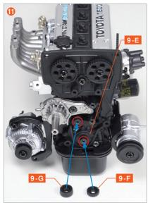
Fit the **Timing Belt Idler 9-G** and the **Crankshaft Timing Pulley 9-F** onto the upper and lower screw pegs of **9-E** respectively.
