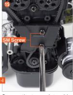
Secure the two points with SP screws.
