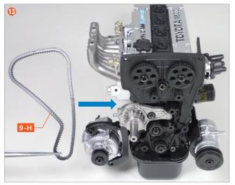
Fit the **Timing Belt 9-H** around the four pulleys on the front of the engine.
