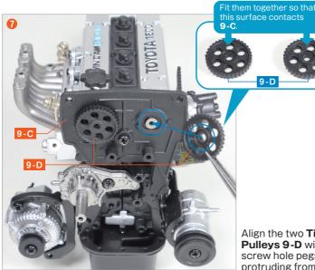
Align the two Timing Belt Pulleys 9-D with the screw hole pegs protruding from 9-C.
