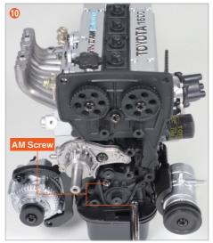
Secure the two points with AM screws.
