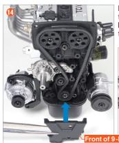
Fit the screw holes on the back of the **Timing** Belt Cover 29-I onto the pegs of 6-A.
