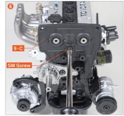
Secure the central lower screw hole with an SM screw.
